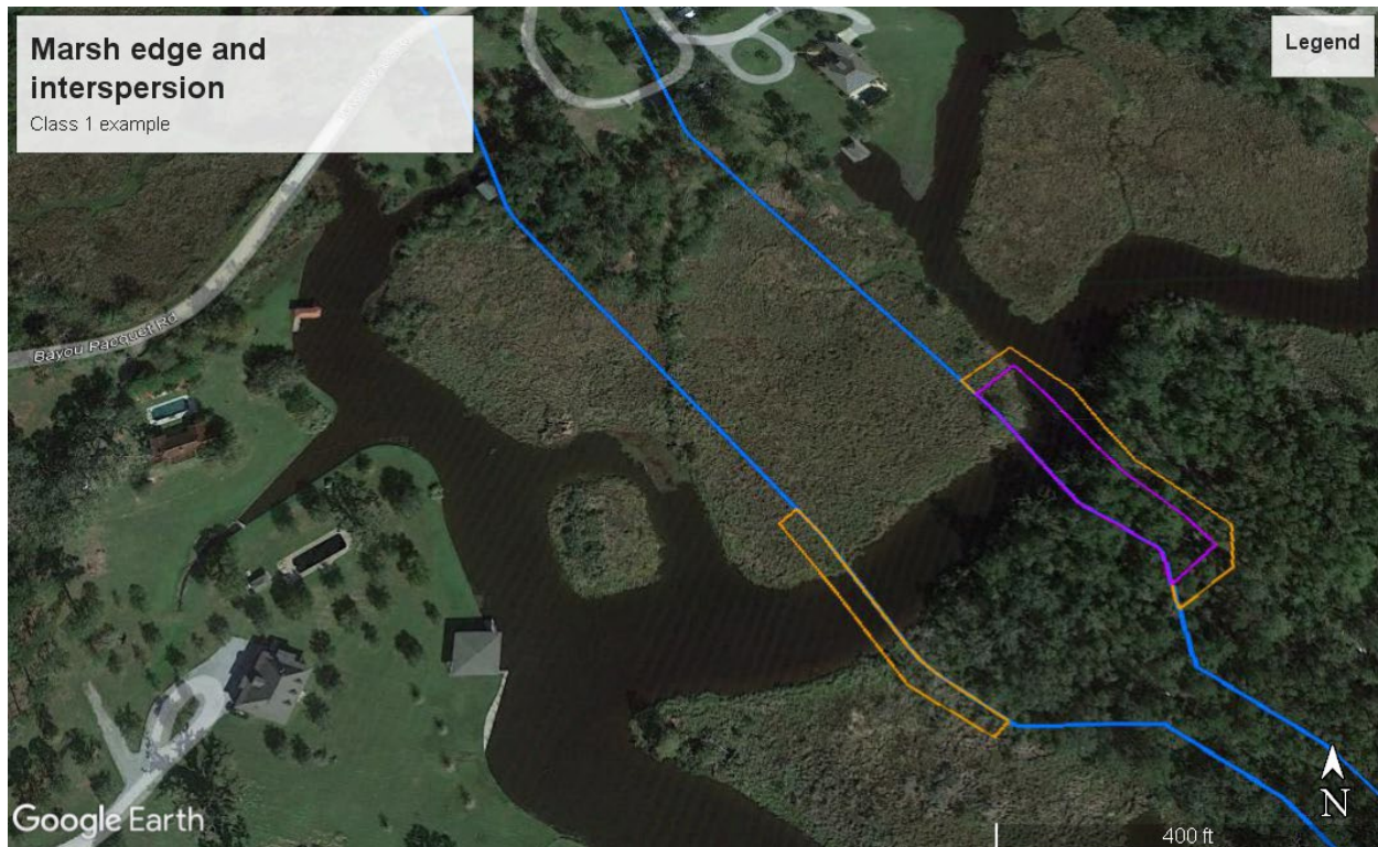
Figure 3. Marsh Interspersion on St. Tammany Project Private lands. Blue lines represent levee footprint and orange and purple lines represent staging areas.
