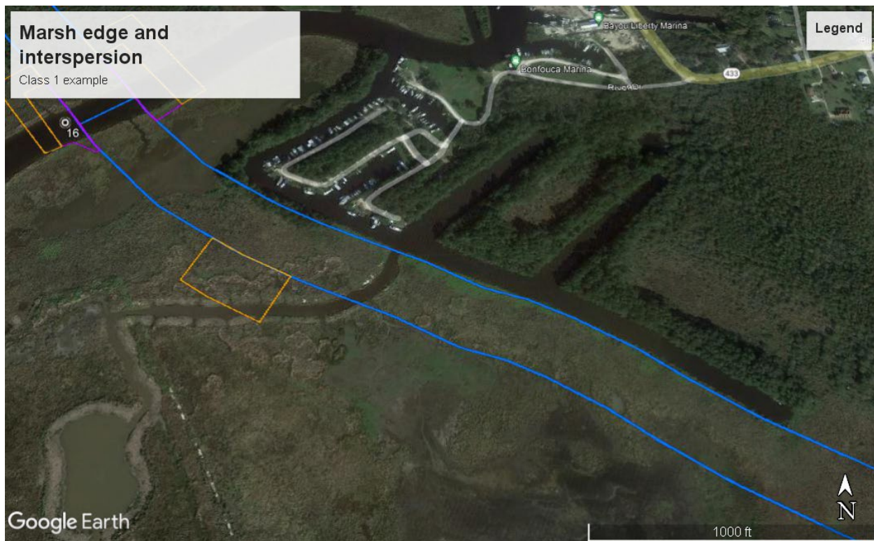
Figure 1. Marsh interspersions on St Tammany Project Big Branch Marsh National Wildlife Refuge land. Blue lines represent levee footprint and orange lines represent staging areas.
